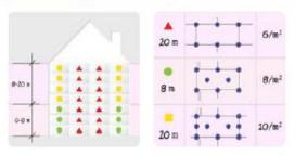
The selection of correct type and length plastic anchor must be selected according to substrate, the type and thickness of thermal insulation plate, the thickness of adhesive and the thickness of plaster. The spot can be applied after the adhesion drying (24 – 28 hours).
